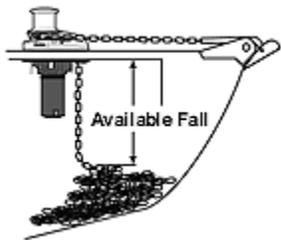
Vertical windlasses provide aesthetic value and offer the added security of the anchor rode making a 180° wrap around the gypsy. The inherent design of the vertical windlass requires at least 12"/ 30cm of fall. This is to allow gravity to properly self-tail the anchor rode through a 90° vertical turn into the anchor locker. Additionally, nylon line is lightweight and a short fall in a vertical windlass system might prevent the rode from feeding properly into the locker
